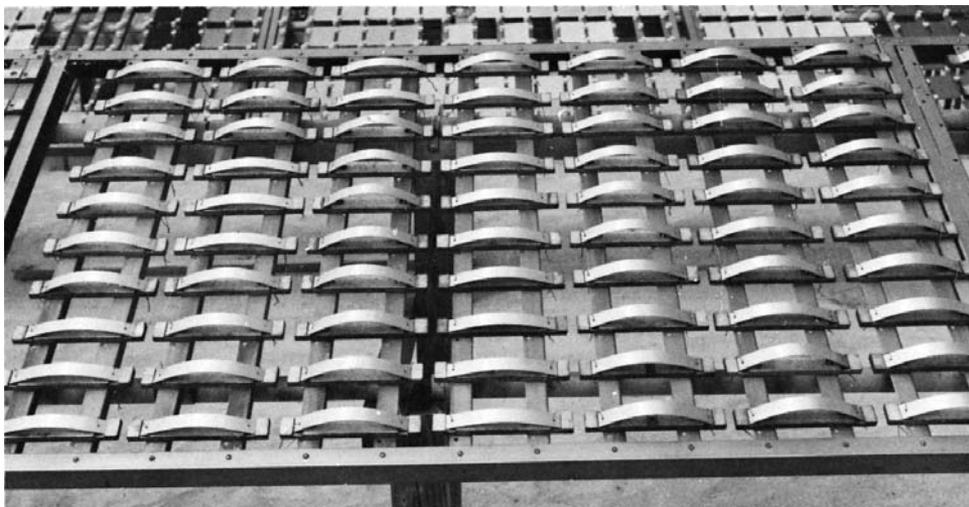
FIG. 4 Bent-Beam Specimens on Atmospheric Exposure Rack
